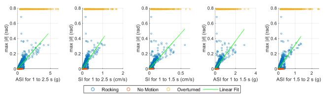
Figure 5. Rotational displacement due to rocking vs. intensity measures for all M-R pairs.
