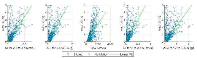
Figure 4. Horizontal displacement due to sliding vs. intensity measures for all M-R pairs.
