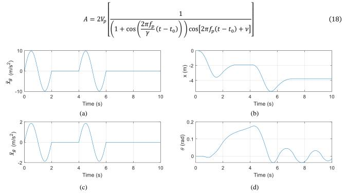
Figure 2. Pure sliding response of rigid block of R = 1.12 m,  $\mu_s = 0.3$ , and  $\mu_k = 0.2$ : (a) input base acceleration, and (b) displacement response. Pure rocking response of rigid block of R = 3.29 m,  $\mu_s = 1.3$ , and  $\mu_k = 1.2$ : (c) input base acceleration, and (d) angular displacement response.
