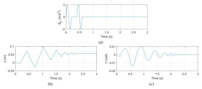
Figure 3. Slide-rocking response of rigid block of R = 2.06 m,  $\mu_s = 0.3$ , and  $\mu_k = 0.2$ : (a) input base acceleration, (b) displacement response, and (c) angular displacement response.
